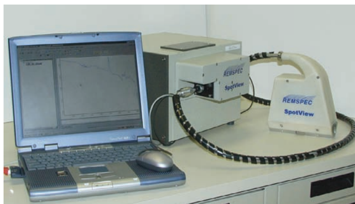
Figure 1 SpotView system, including the mid-IR spectrometer with fiber optic cable attached to the sampling head (at right) and the laptop computer used for operation.
