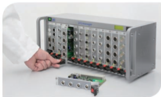
Easy „on-the-fly“ change of the slide-in modules
