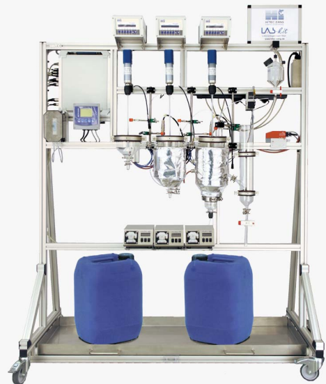
Laboratory clarification unit with pH, turbidity and foam sensors, stirred tanks in continuous operation
