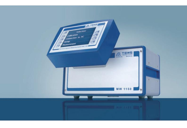
The MW 1150 is designed as a small compact laboratory instrument or atline instrument. It is based on the MW 11xx technology which allows readings within milliseconds to obtain sensor values quickly and reliably. The backlit 5.7" (14,5 cm) monitor displays the results - up to 250 readings can be stored in the system memory, atline applications use the standard 4-20mA interface to transfer values to a PLC. There are ports for a P 1150-type printer and various temperature sensors.
