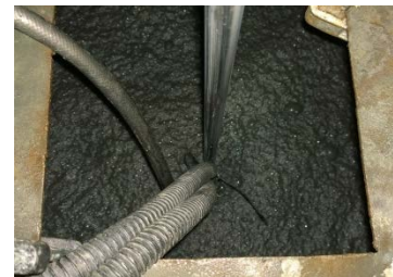
Figure 2. Imaging hardware submersed 1.5m beneath the froth layer of the mineral flotation cell
