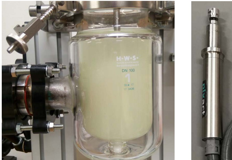
a) Figure 1. a) Emulsion of diesel droplets in water in a 1-liter laboratory reactor. b) Pixact imaging probe with a 32 mm measurement head and a 10 mm measurement gap.
