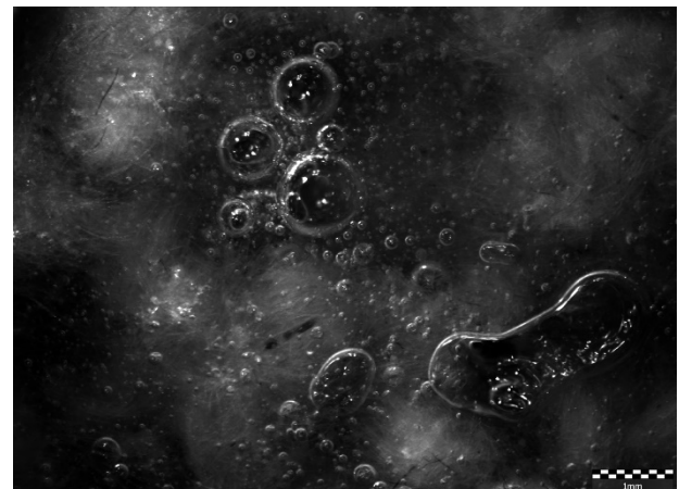
Figure 2. Oxygen bubbles near the reactor inlet. The image shows that dispersion has been far from optimal. 1 mm scale bar.
