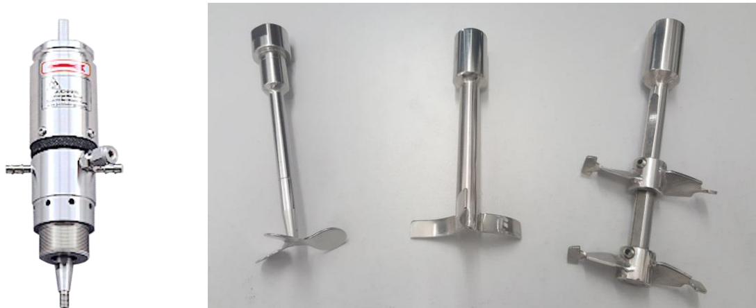
Figure 3: Left: Magnetic stirrer head. Right: Excerpt from stirrer geometry choices
