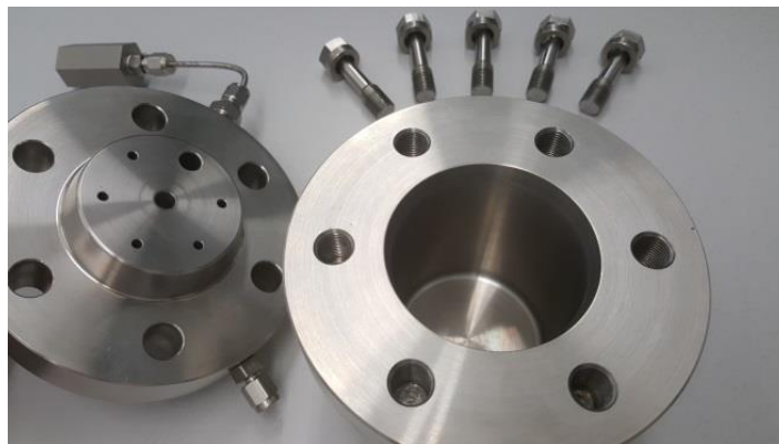
Figure 2: Opened HiClave reactor: purely metallic sealing
